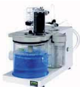
Scrubber K-415 (condensation-neutralization-adsorption unit)
