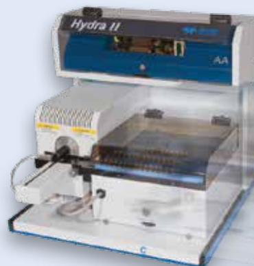
Hydra II c Atomic Absorption Detection – Direct analysis of Solid and Semi Solids
